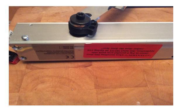
FOR EASE OF SECURING TO THE DOOR CLOSE THE DOOR SPEED VALVE AND PULL ARM LEVEL WITH THE CLOSER. ONCE INSTALLED OPEN DOOR SPEED VALVE TO GIVE DESIRED CLOSING SPEED
