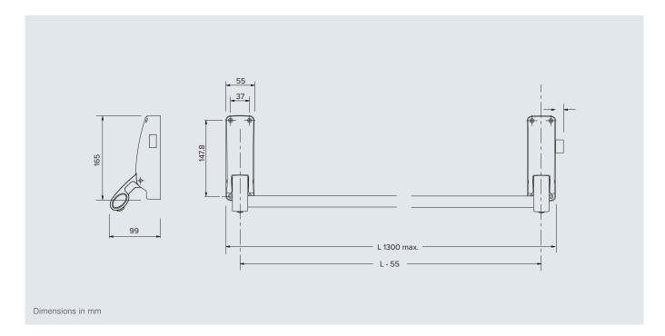
Minimum width of stiles 78mm for 13mm rebates and 90mm for 25mm rebates.
